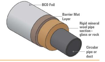
**ACOUSTEK WRAP** consists of 45kg/m3 stone wool lamella strips which are bonded to a mass barrier membrane. The mass barrier incorporates reinforced Bright Class O aluminium foil to the exposed side.
