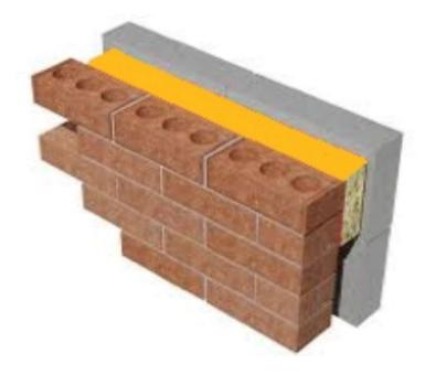
**Acoustic –U-Spec Cavity Barriers** also help to meet the acoustic requirements of Approved Document E (England & Wales) and Section 5 (Scotland) by minimising flanking sound transmission along cavity walls.
